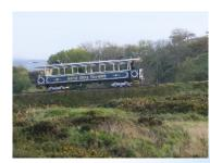
The **Great Orme Tramway** first opened in 1902, and is the only remaining cable-operated street tramway in Great Britain. The tram cars are the original vehicles.
